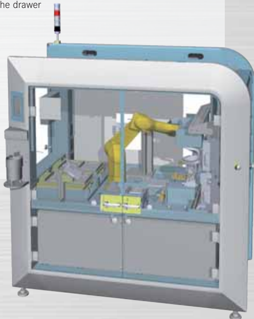
Component storage and supply by means of an oscillating conveyor. Type recognition and rotary orientation recognition is performed by a camera system buffering of the finished components in the drawer
