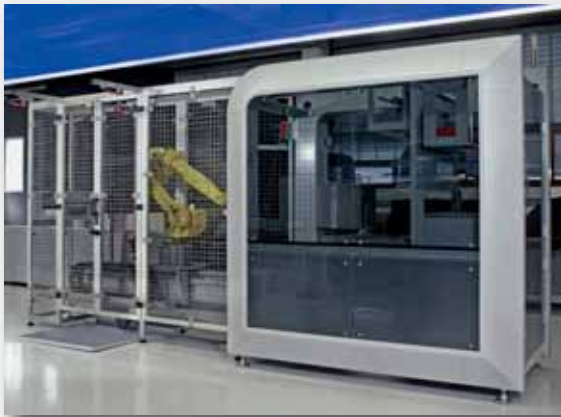
SRZ 300/10-2P with 7th supplementary axis, interlinking of three machine tools
